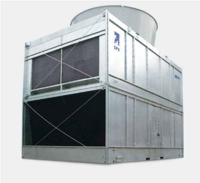
MARLEY NCWD HYBRID CROSSFLOW COOLING TOWER Coil-based, factory-assembled hybrid cooling tower designed to reduce visible plume and enhance water conservation. Tower capacity from 298 to 498 tons per cell.
