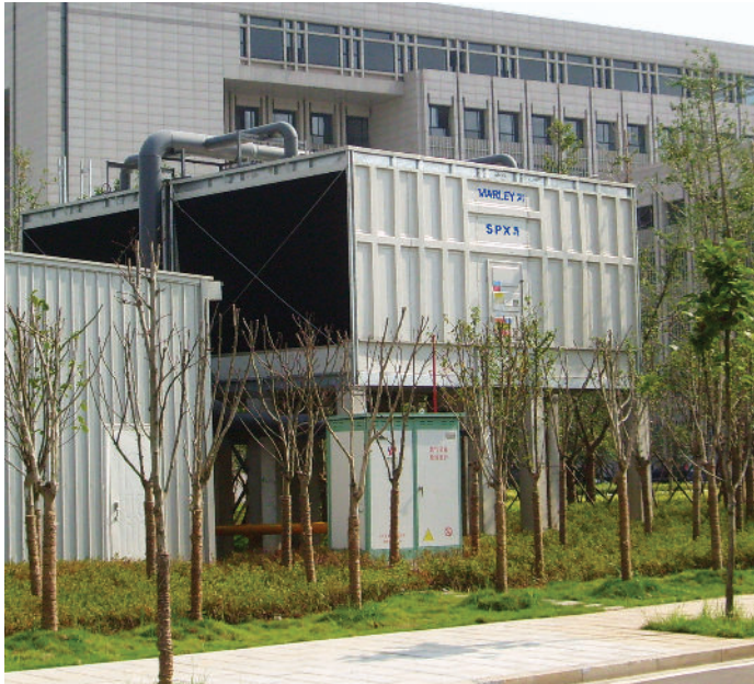
MARLEY NC FIBERGLASS CROSSFLOW COOLING TOWER Fiberglass and galvanized steel, field-erected cooling tower designed to serve air conditioning and refrigeration systems as well as light to medium industrial process loads on clean water. Stainless steel structure option. Tower capacity from 101 to 1,455 tons per cell. CTI Certified. Not available in the US, Canada or Europe.
