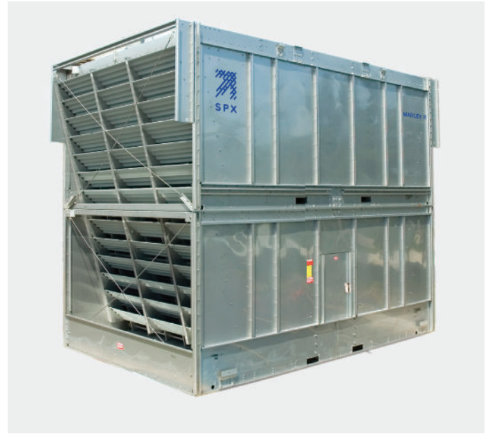
MARLEY NC® ALPHA CROSSFLOW COOLING TOWER Splash-fill design for use at high temperature or where poor water quality prevents the use of film fill. Factory assembly and G-235 galvanized steel construction are standard. Stainless steel option expands applications. Tower capacity from 290 to 2,700 gpm per cell.
